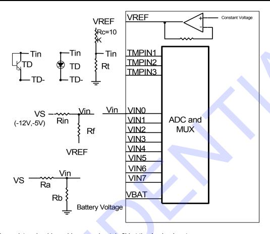
Note: The resistor should provide approximately 2V at the Analog Inputs.
