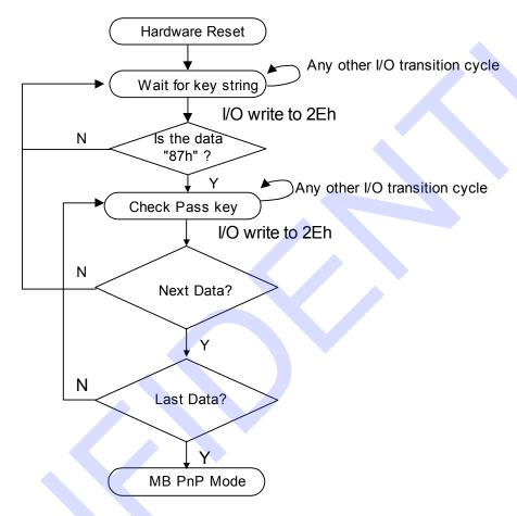
There are three steps to completing the configuration setup: (1) Enter the MB PnP Mode; (2) Modify the data of configuration registers; (3) Exit the MB PnP Mode. The undesired result may occur if the MB PnP Mode is not exited properly.
