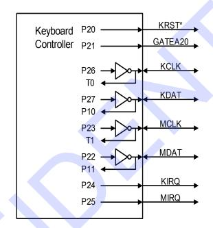
Figure 9-10. Keyboard and Mouse Interface
